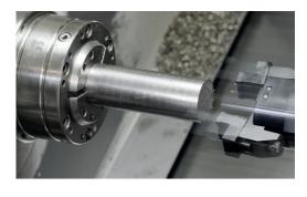
Move the bar gripper in Z direction off the bar and start machining.
