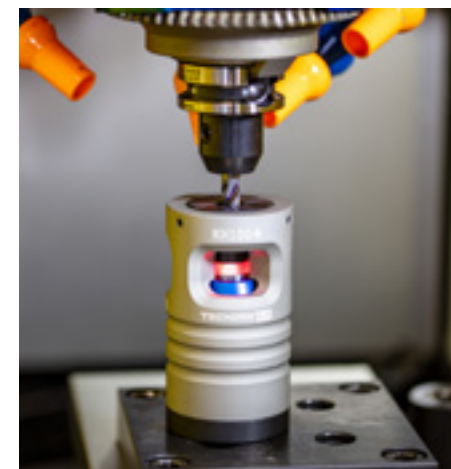
Determining the zero point
