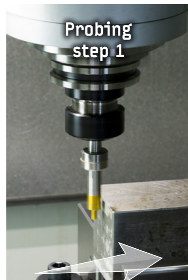
1. The edge finder body can be tilted out from the axis' centre by a gentle tip of the finger and is out-of-the-round.
